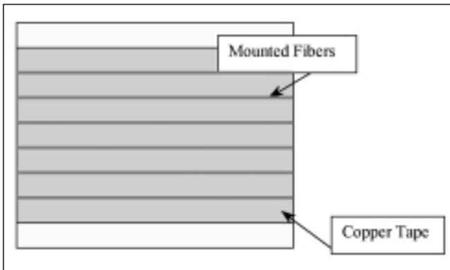
Fig. 3. Copper tape with fibers, bent 180°.
