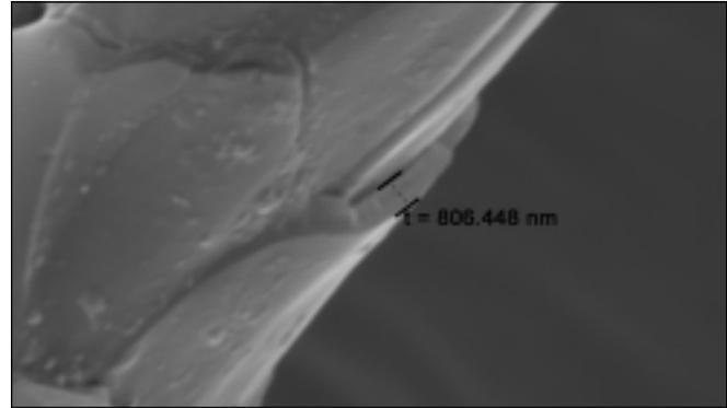
Fig. 2. Fiber prepared for longitudinal CSH measurement (10,000x magnification).
