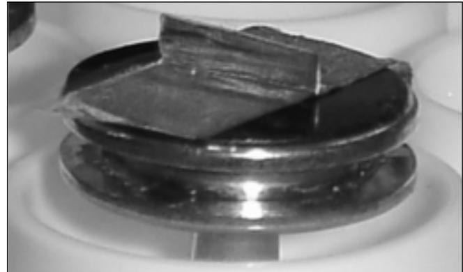
Fig. 4. Animal fiber bent over copper tape showing areas where sequential vertical scale height can be measured (223x magnification).
