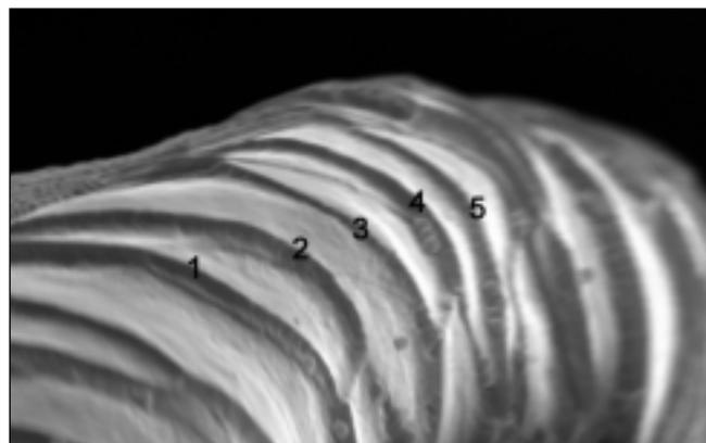
Fig. 7. Wool fiber image with NIST internal standard and scale sequence (6,840x magnification).
