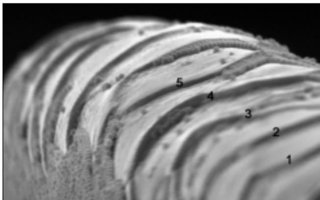
Fig. 6. Cashmere fiber with NIST internal standard and scale sequence (6,490x magnification).
